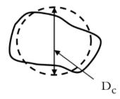
Fig. 3. Circle-equivalent diameter of the equal-area
