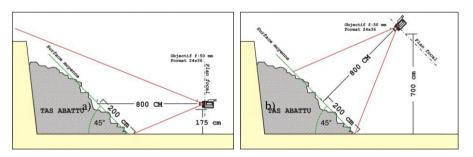
Fig. 1. The problem of parallax in the photographic sampling (Tessier, 2008) a) Parallax error (b) Parallax well controlled
